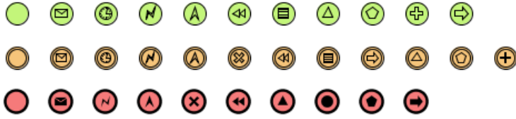
Start, intermediate and end events with different kinds of triggers and results
