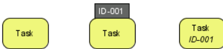
Different looks of a BPMN task when ID is not shown, ID is shown as label and ID is shown below caption
